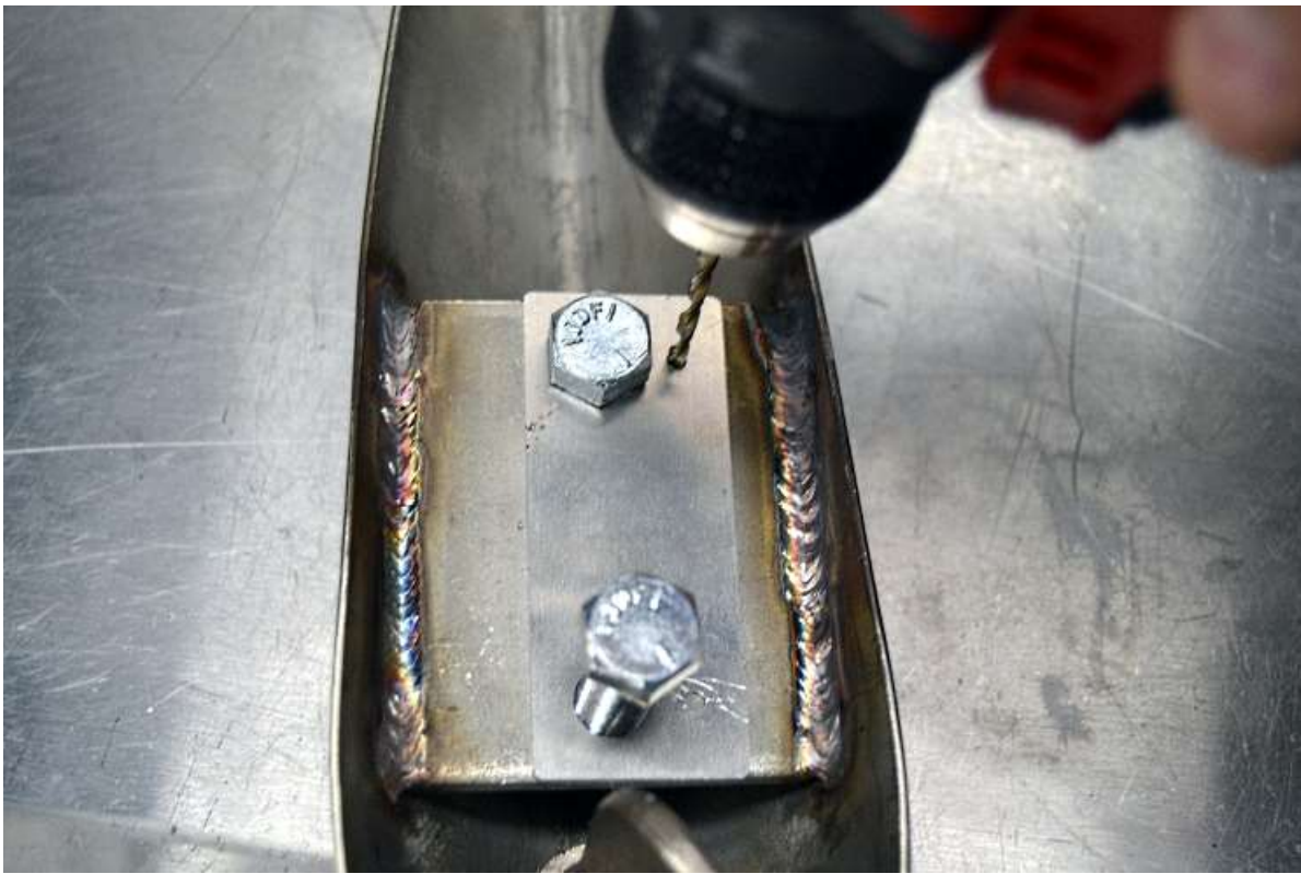
Use the short screws and drill template provided to drill \frac{1}{8} " holes towards the inside of the overrider. left side shown.
