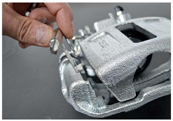
Insert one of the metal clips into the caliper and hold in place.
