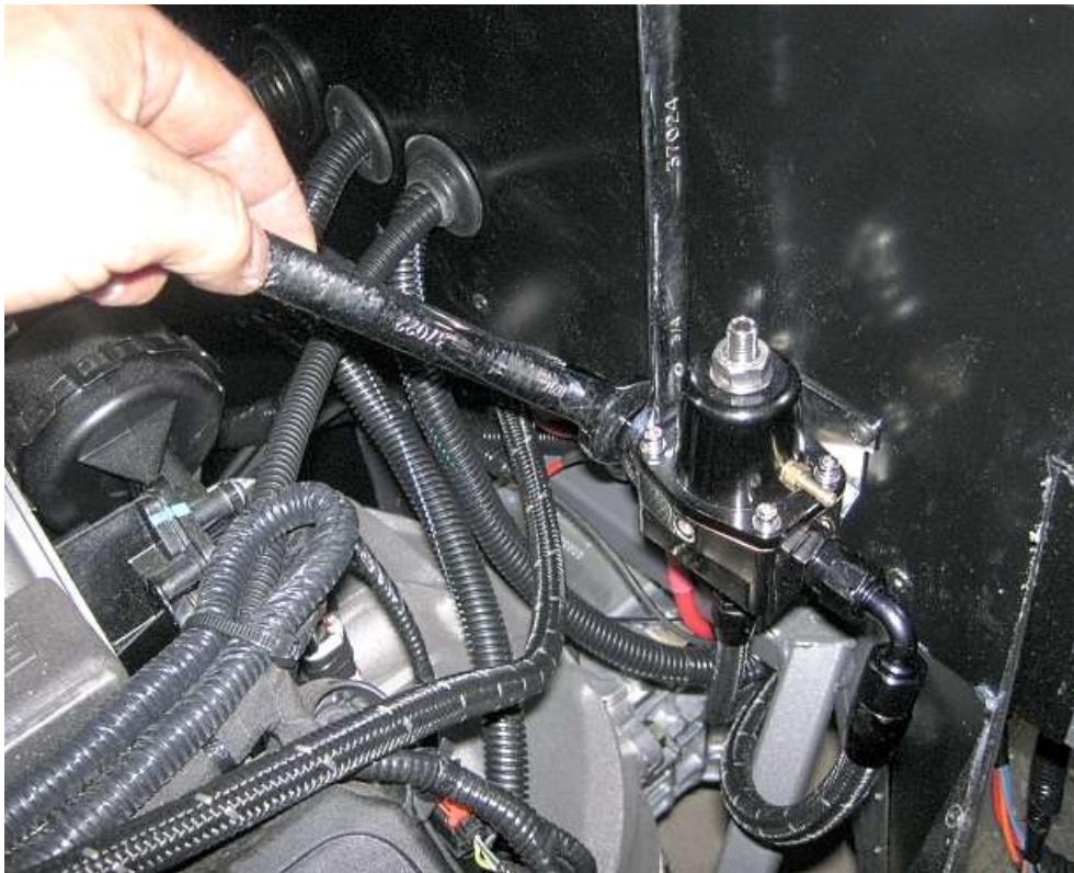
Tighten the fitting on the Regulator using 1\frac{1}{16} " and \frac{3}{4} " wrenches.
