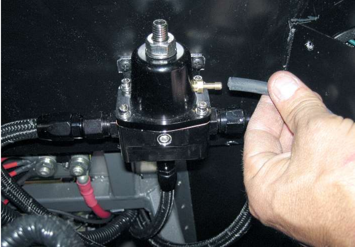
Attach the vacuum line to the intake and regulator if not already done.
