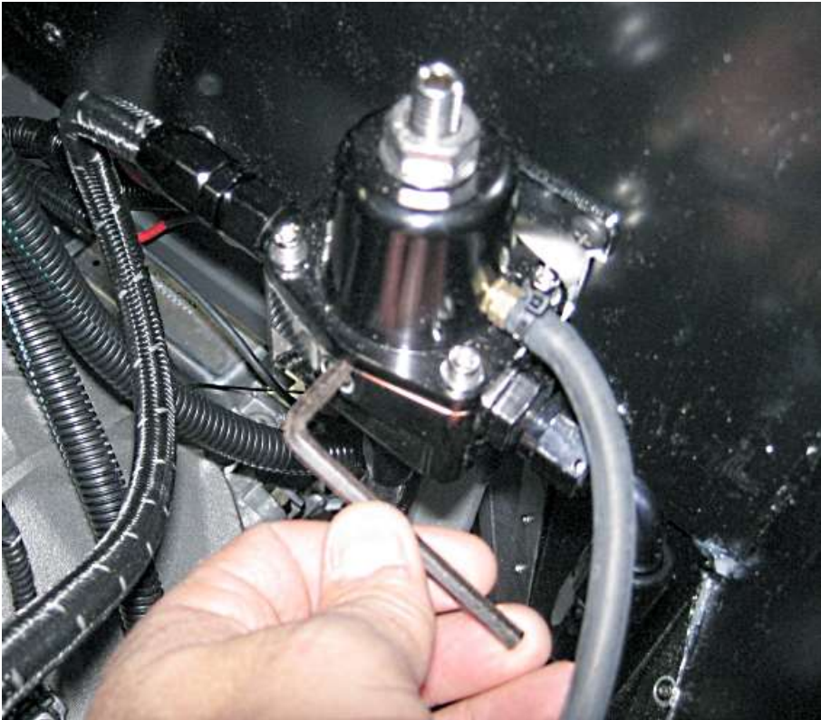
Remove the set screw on the front of the regulator.
