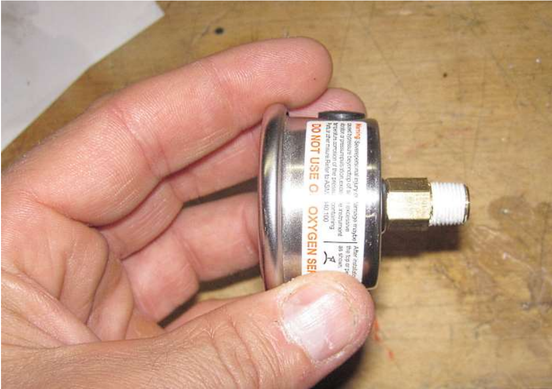
Put Teflon tape on the fuel pressure gauge threads.
