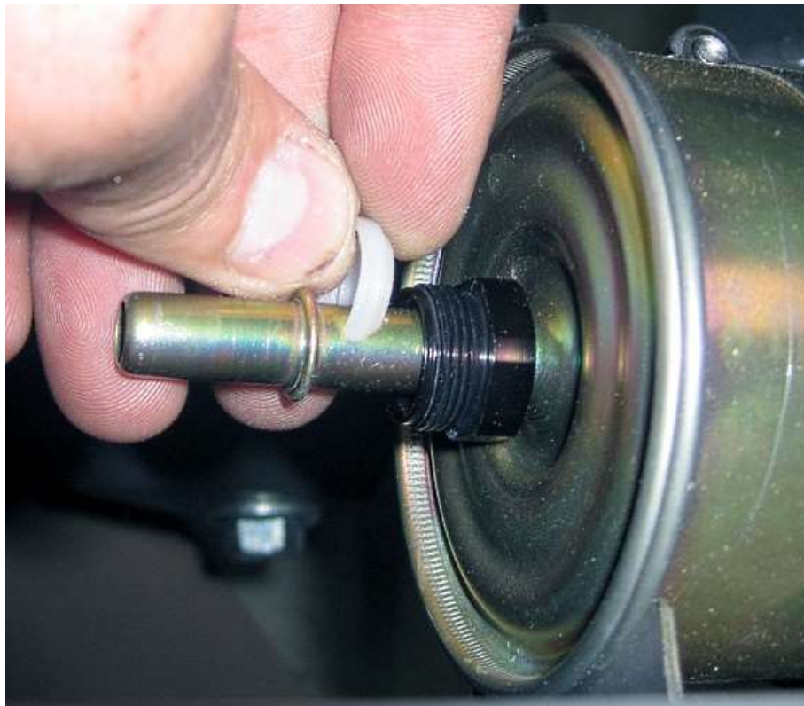
Put the small white plastic piece behind the bead on the filter with the curved part towards the black fitting end.
