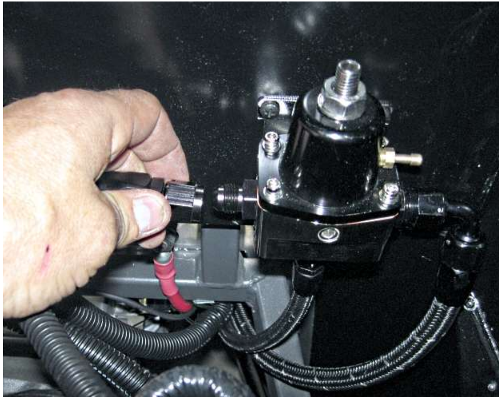
Screw the fuel line that goes to the engine to the regulator.
