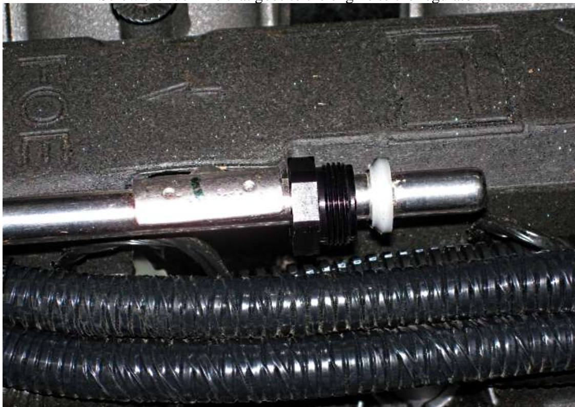
Slide the black end and small white plastic piece behind the bead on the of the fuel rail on the engine
