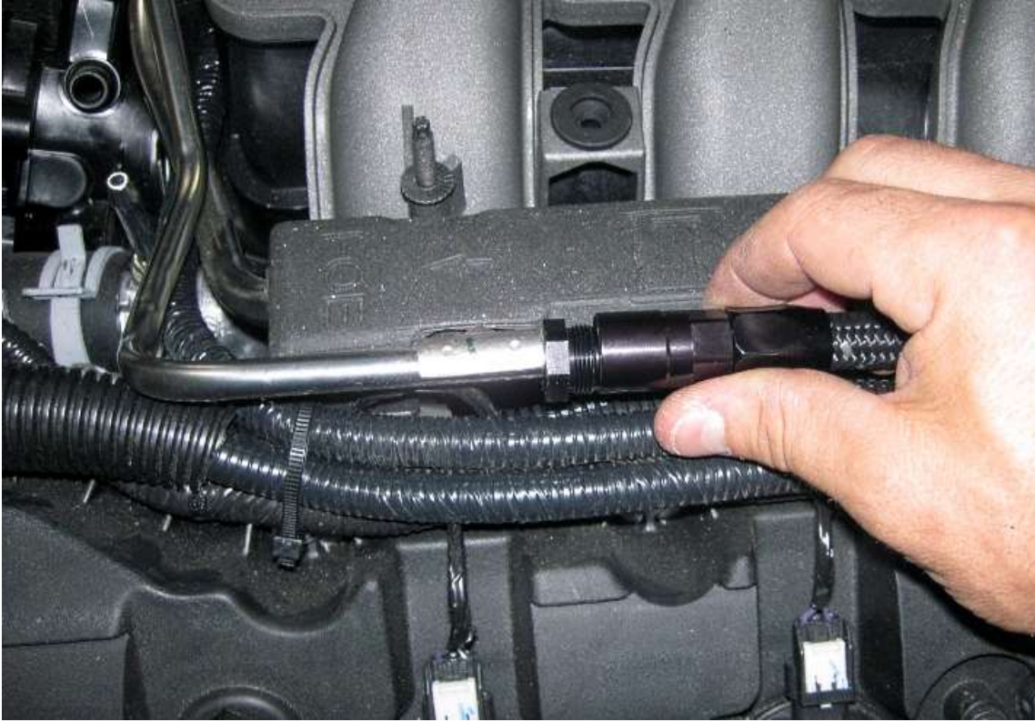
Screw and tighten the end of the fitting onto the hose using 1\frac{1}{16} " and \frac{3}{4} " wrenches.
