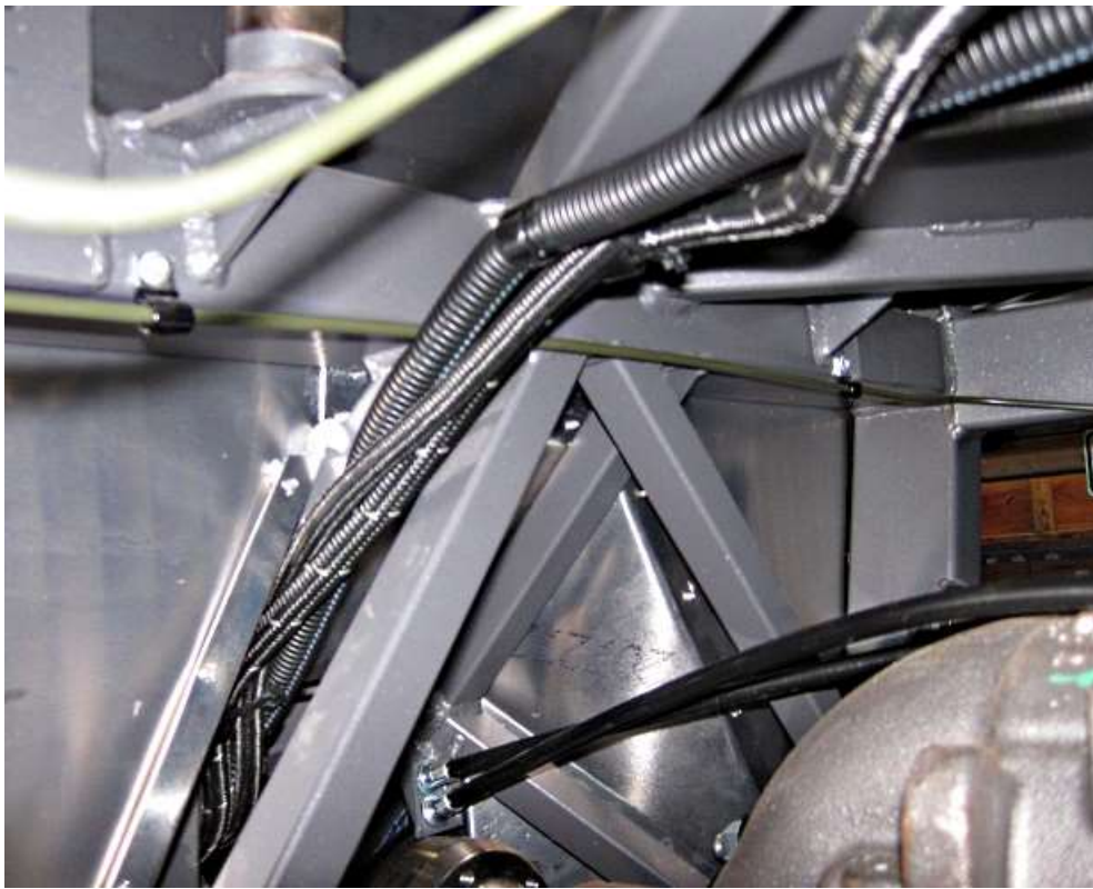
Run the lines up and over the rear axle.
