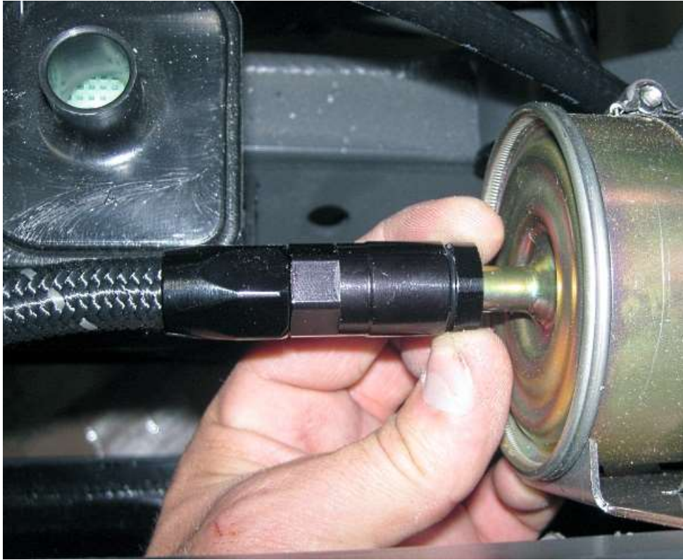
Push the send hose onto the end of the filter.
