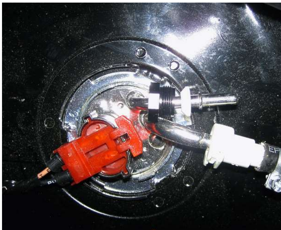
Push the white plastic piece on the tube behind the bead.
