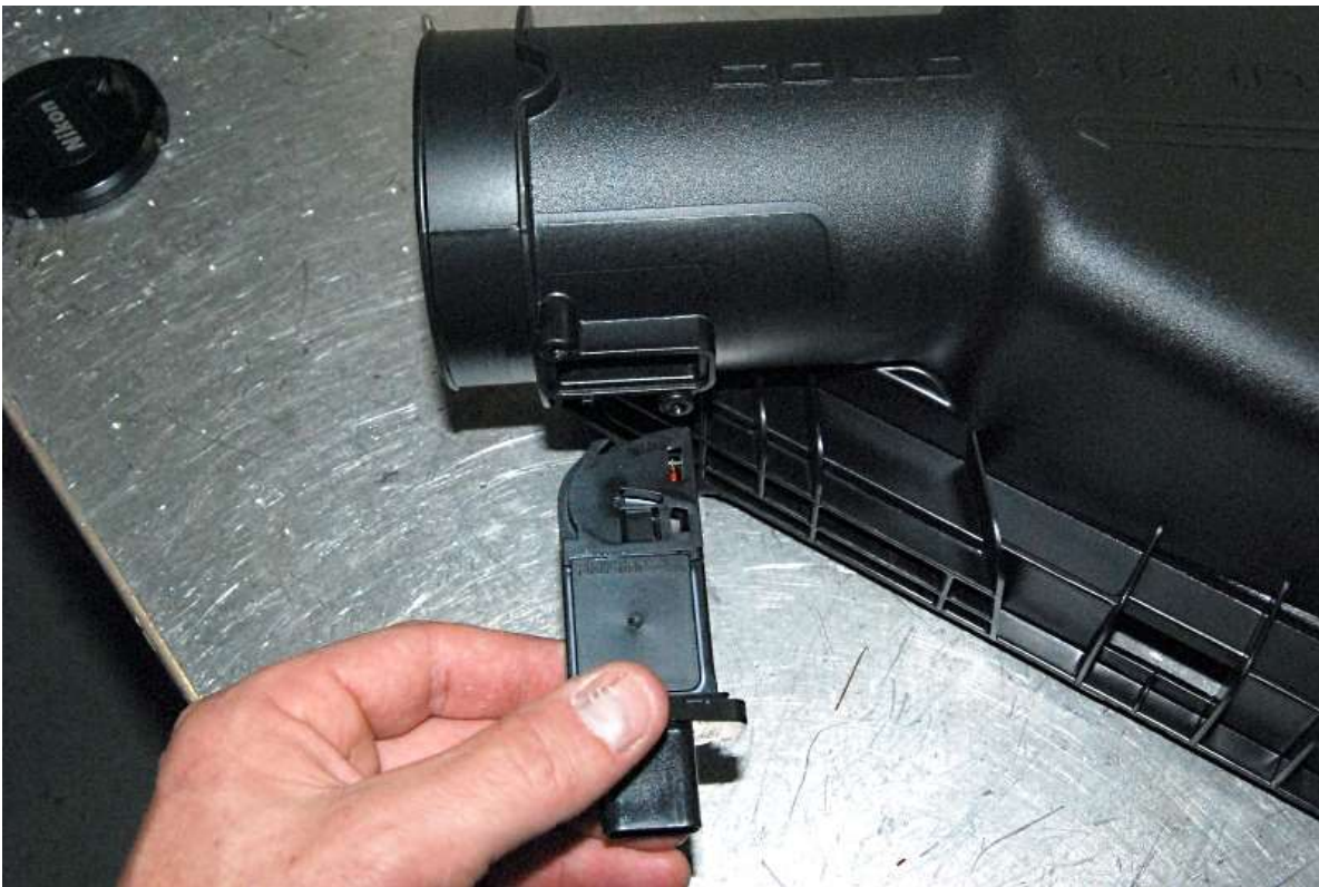
Remove the sensor and note the direction of the curved part of the sensor, on the engine side.
