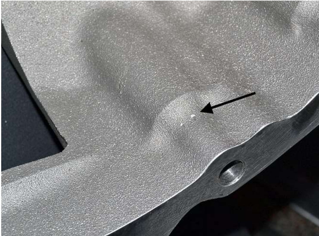
These marks show the interference of the flywheel and bellhousing.
