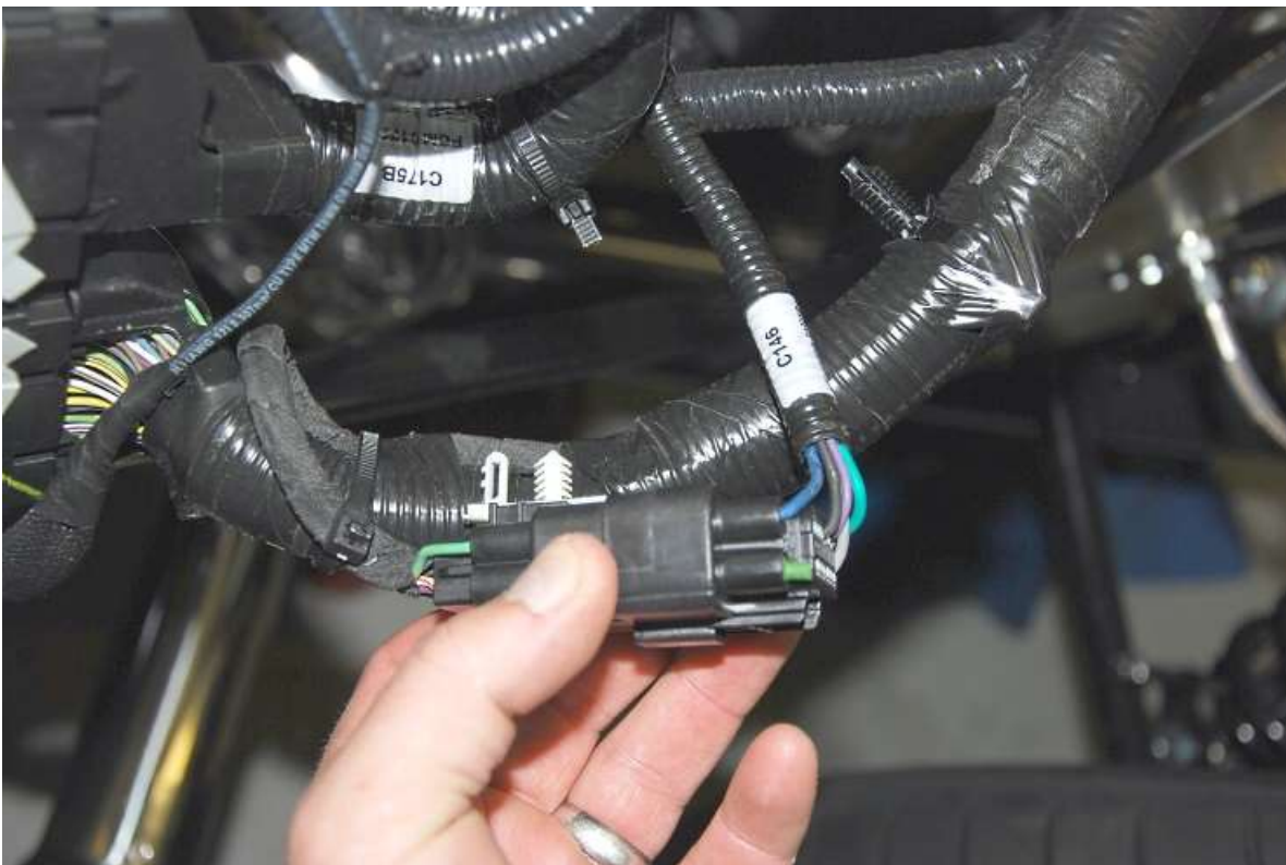
Connect the 16 pin Engine harness plug to the control pack plug next to the computer.
