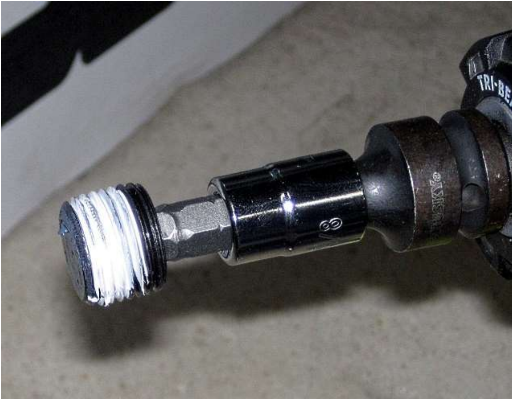
Put Teflon tape onto the plugs included with the oil pan.
