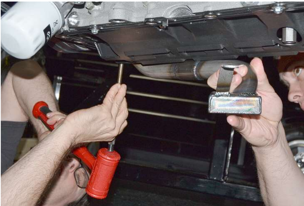
Insert the pick-up into the pump through the windage tray, you may need to use a flathead screwdriver and plastic hammer on the pick-up flange on the pump so that it fully seats.
