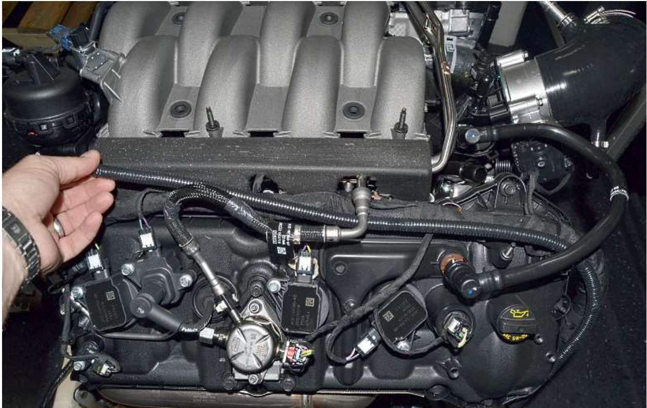
Run the Alternator/Mass Air long harness leg across to the engine with the engine harness then to the back of the engine.
