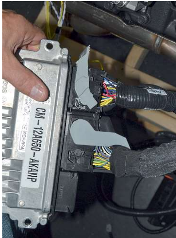
Connect Engine harness plug to the computer.
