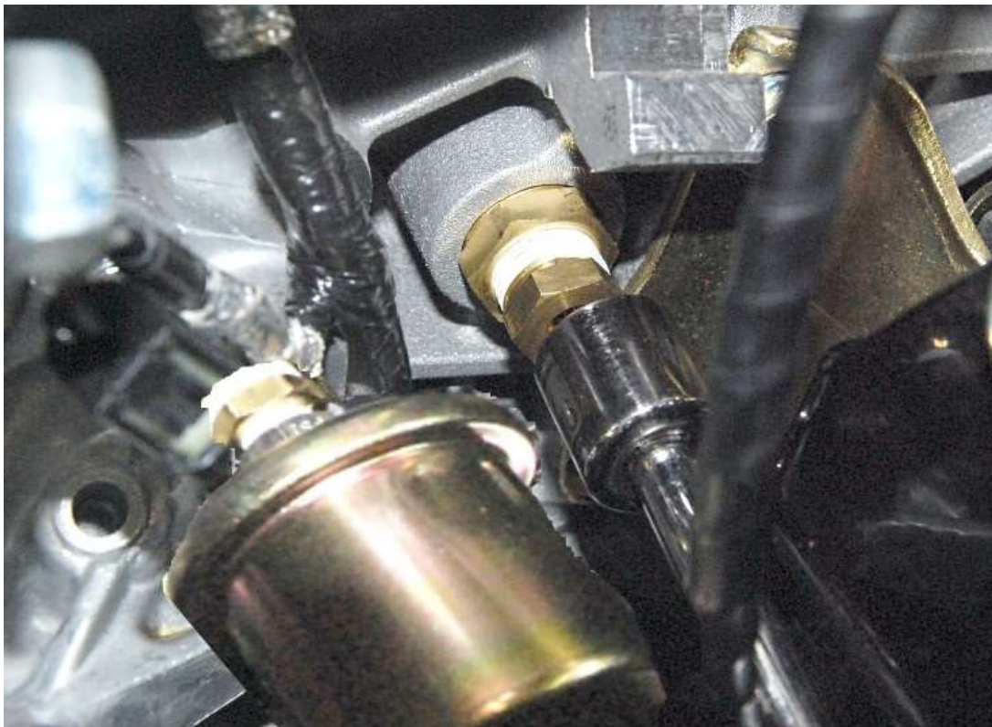
Screw the adapter into the larger adapter on the block.
