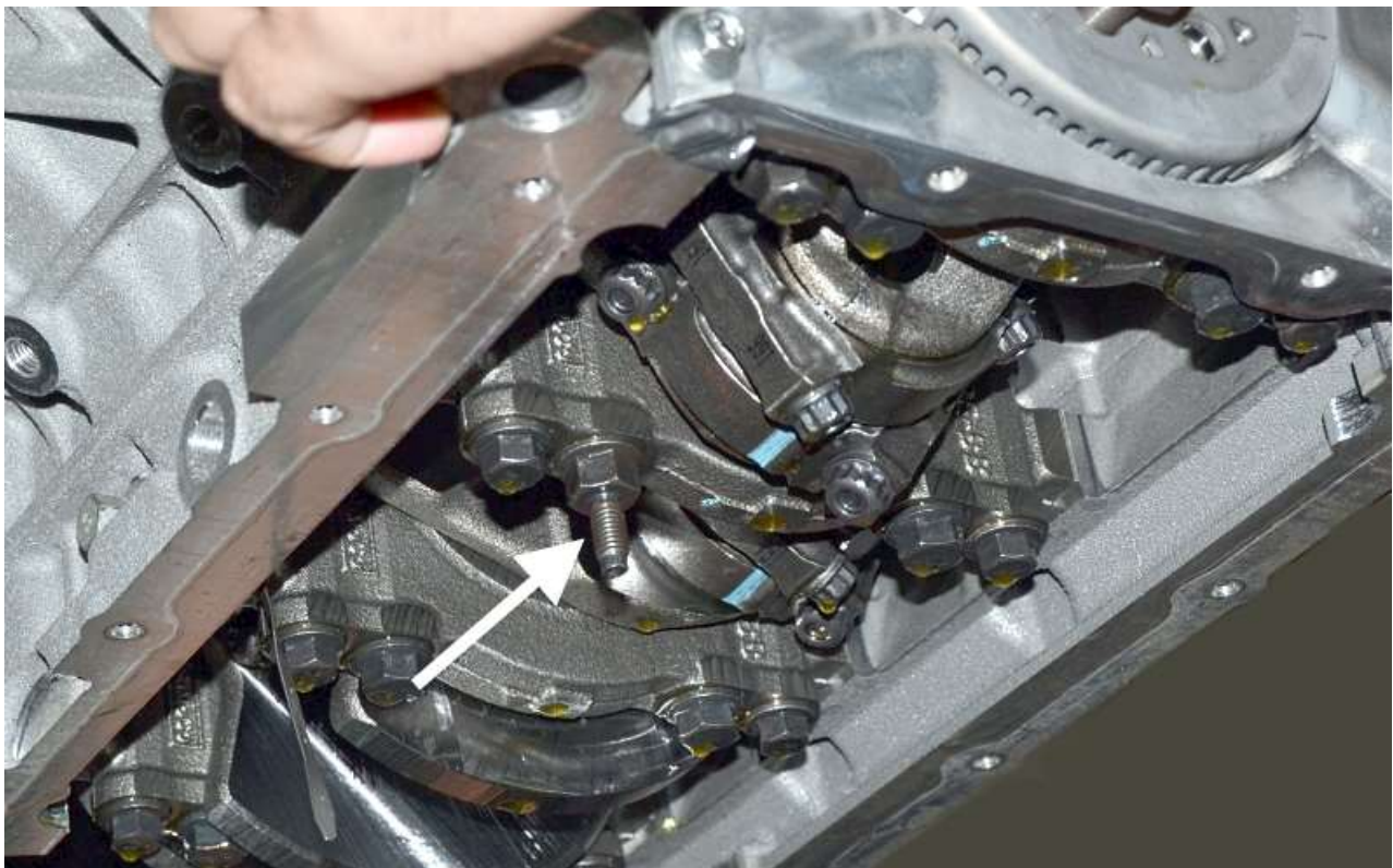
Install the new main cap bolt with the threaded stud that is included with the pick-up and torque to 48 Lbft (65Nm) + 90° turn.
