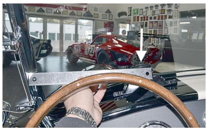
Move the heater duct so that the center of the duct end is centered in your line of sight looking out of the car. This is approximately 11" from the inside of the windshield side bar.
