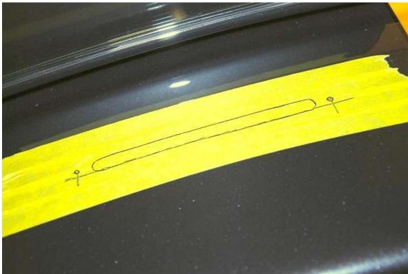
Cut the center of the template and screw holes out then tape it onto the body so that the close side of the hole is on the duct line drawn before and at least one of the screw holes is on the mounting hole line drawn then use a pen and mark the screw holes and duct hole.
