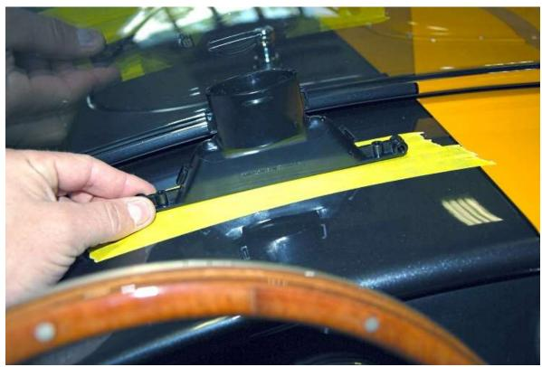
Use one of the plastic defroster ducts and place it upside down on the masking tape in front of the driver. The end of the duct will hit the windshield. This is also the center location where the heater air will hit the windshield.
