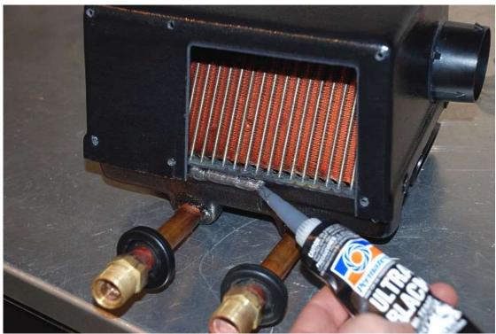
To prevent any air leakage between the heater box and the firewall, use some high temp RTV silicone just above the heater core tubes as shown in the picture below. Make sure you use enough so that it will seal against the firewall.
