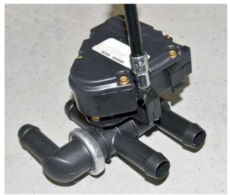
If running a Coyote engine, the cable 2-port control valve cannot be used. A 4-port control valve is needed. This is available from Factory Five. Coolant needs run through the tube for the engine and the 2-port valve does not allow this when off.
