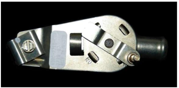
Push the mechanical valve to the off position.
