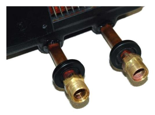
Push the large grommets over the heater core connection nuts onto the tubes. Some WD40 on the grommets may help.
