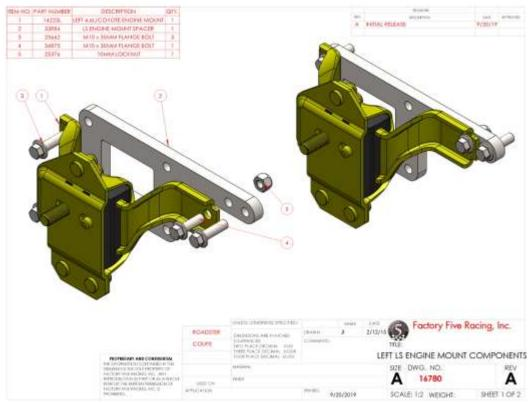
Attach the left side polyurethane mount to the adapter bracket.
