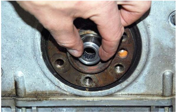
Install the pilot bearing so that it is flush with the stepped area.
