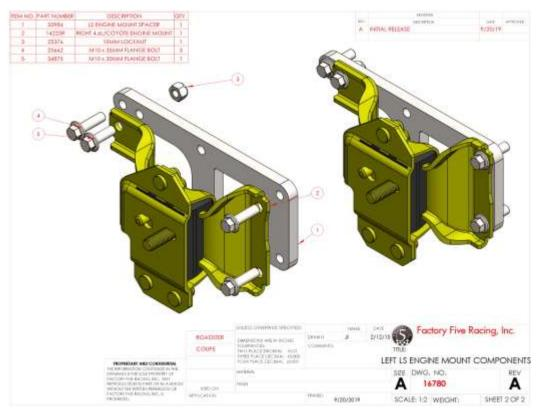
Attach the right side polyurethane mount to the adapter bracket
