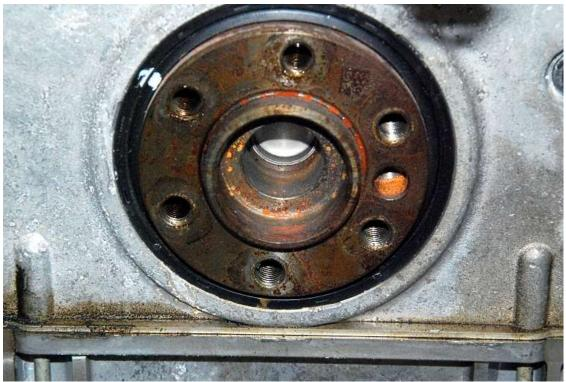
Make sure there is no pilot bearing in the end of the crank shaft already.
