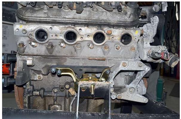
Attach the engine mount to the engine. There are multiple holes to accommodate the different year LS blocks.
