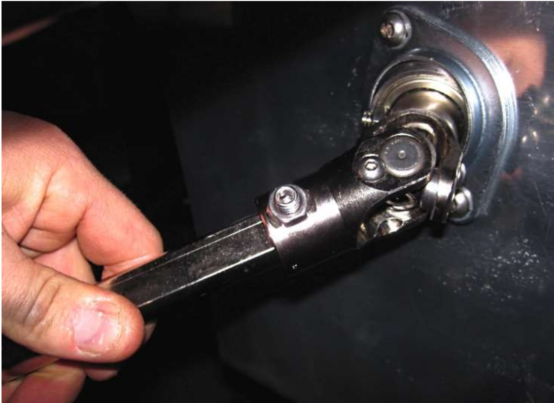
Insert the shaft into the joint on the firewall.
