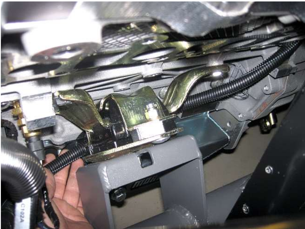
Run the chassis harness wires under the engine mount to keep them away from the header.
