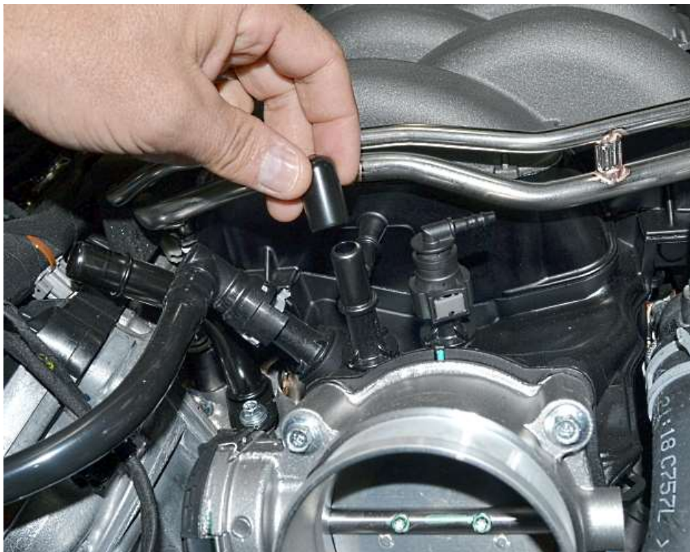
Block off the \frac{1}{2} " large vacuum port just behind the throttle body.
