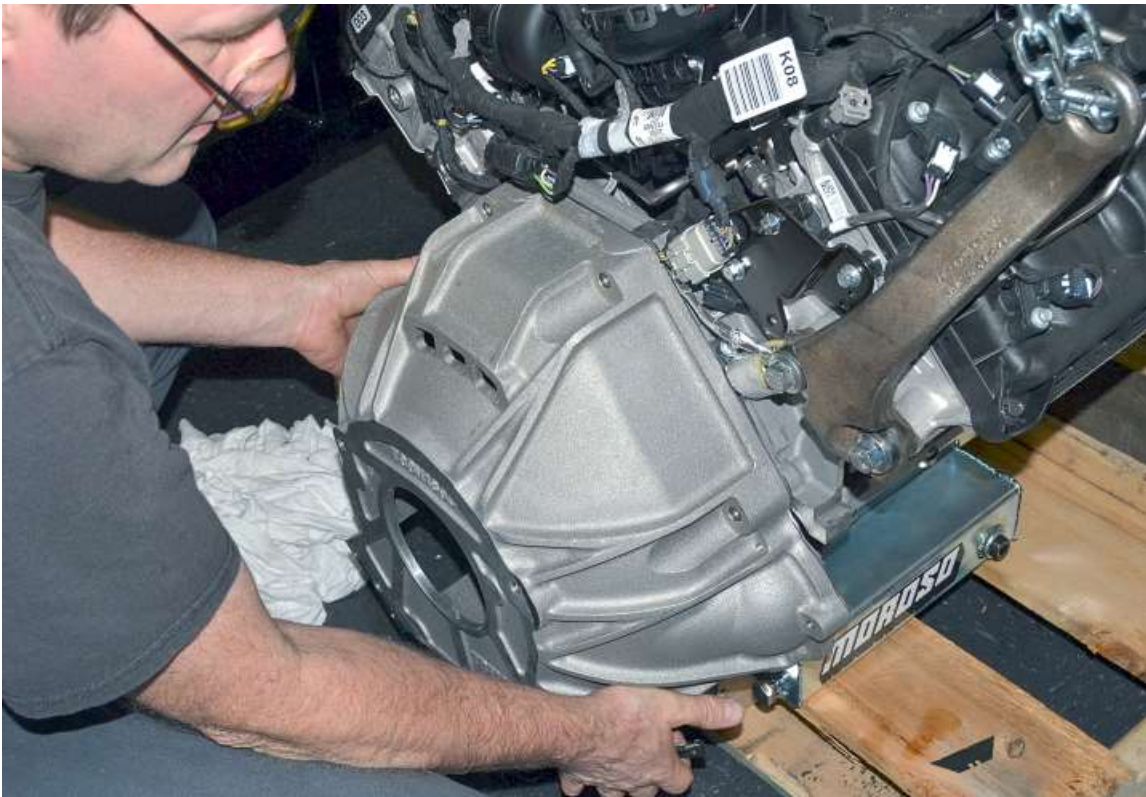
Attach the bellhousing to the engine using a couple of the bellhousing bolts.
