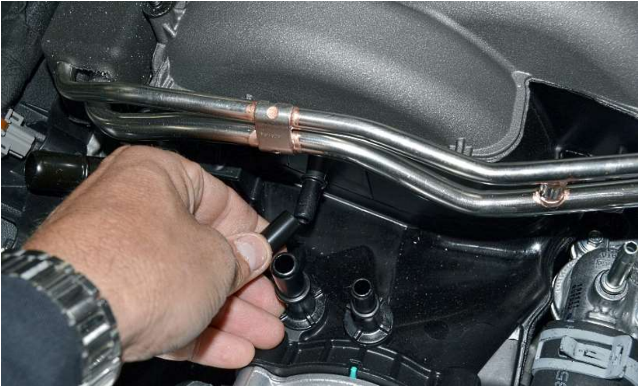
On the front of the intake manifold, push the \frac{3}{8} " Vacuum cap onto the vacuum barb.
