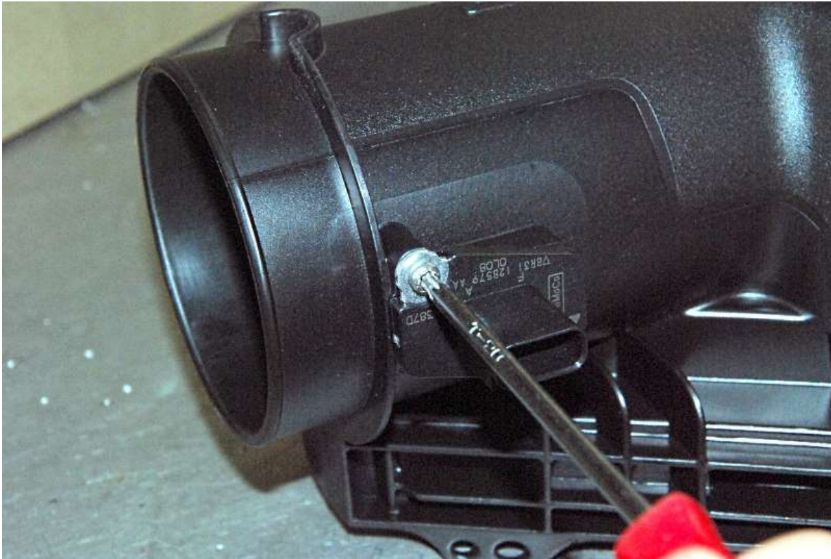
Unscrew the mass air sensor from the Ford intake using a T-20 Torx driver
