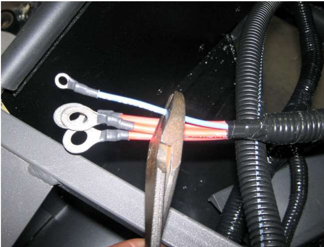
In the chassis harness on the starter wires leg, cut the blue starter wire end off.
