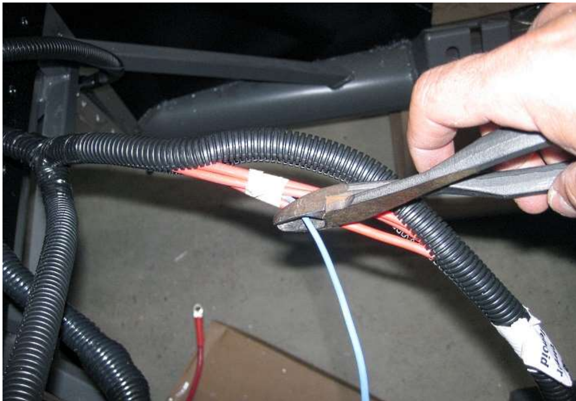
Pull the loom back further down the leg then pull the blue wire out so it does not stick out for the harness and cut it off.
