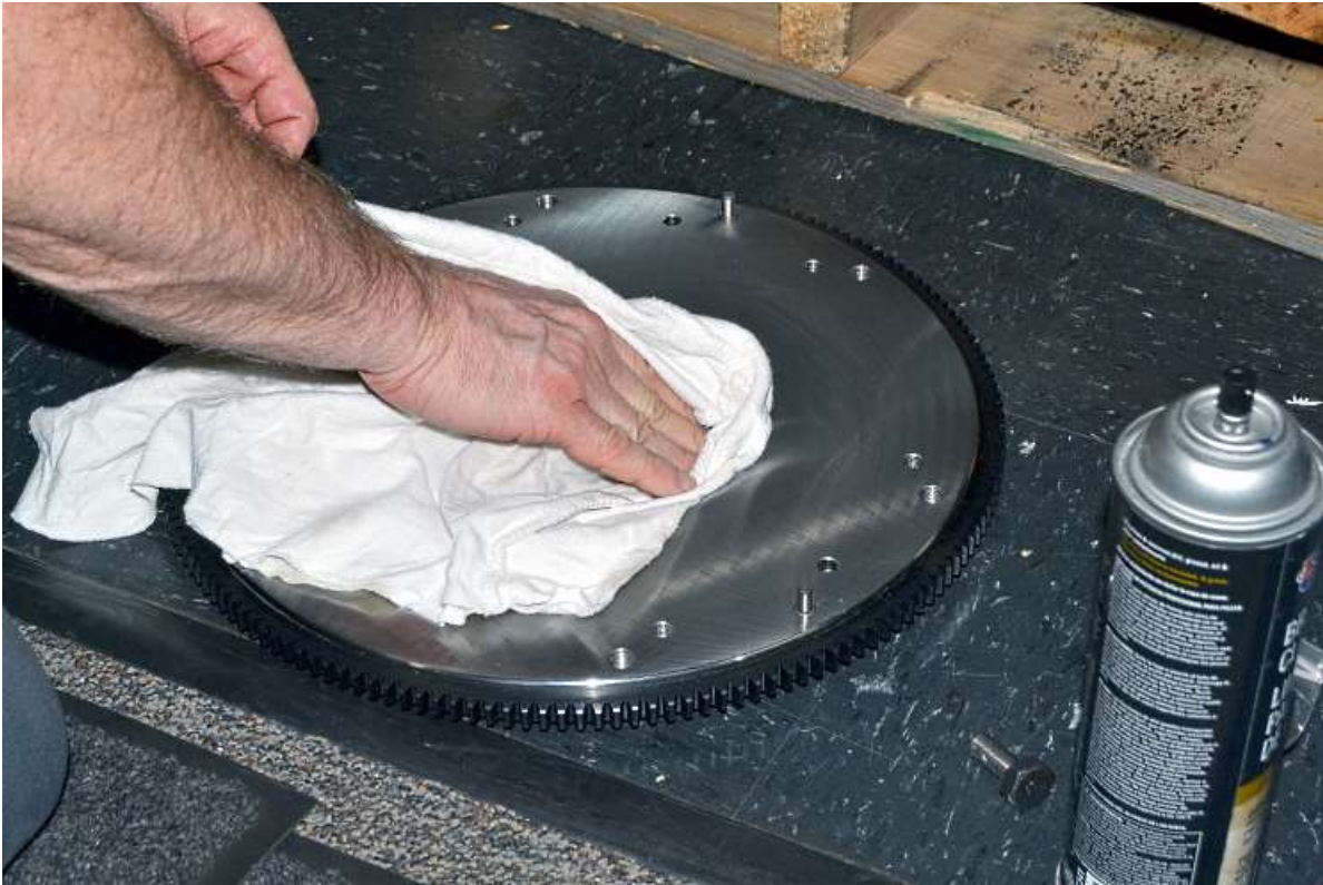
Wipe the flywheel surface off with brake cleaner.
