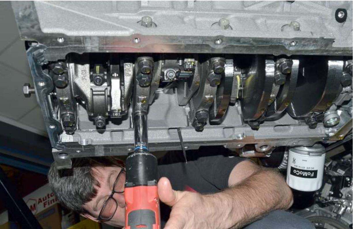
Remove the correct main cap bolt shown in the instructions using a 15mm socket.
