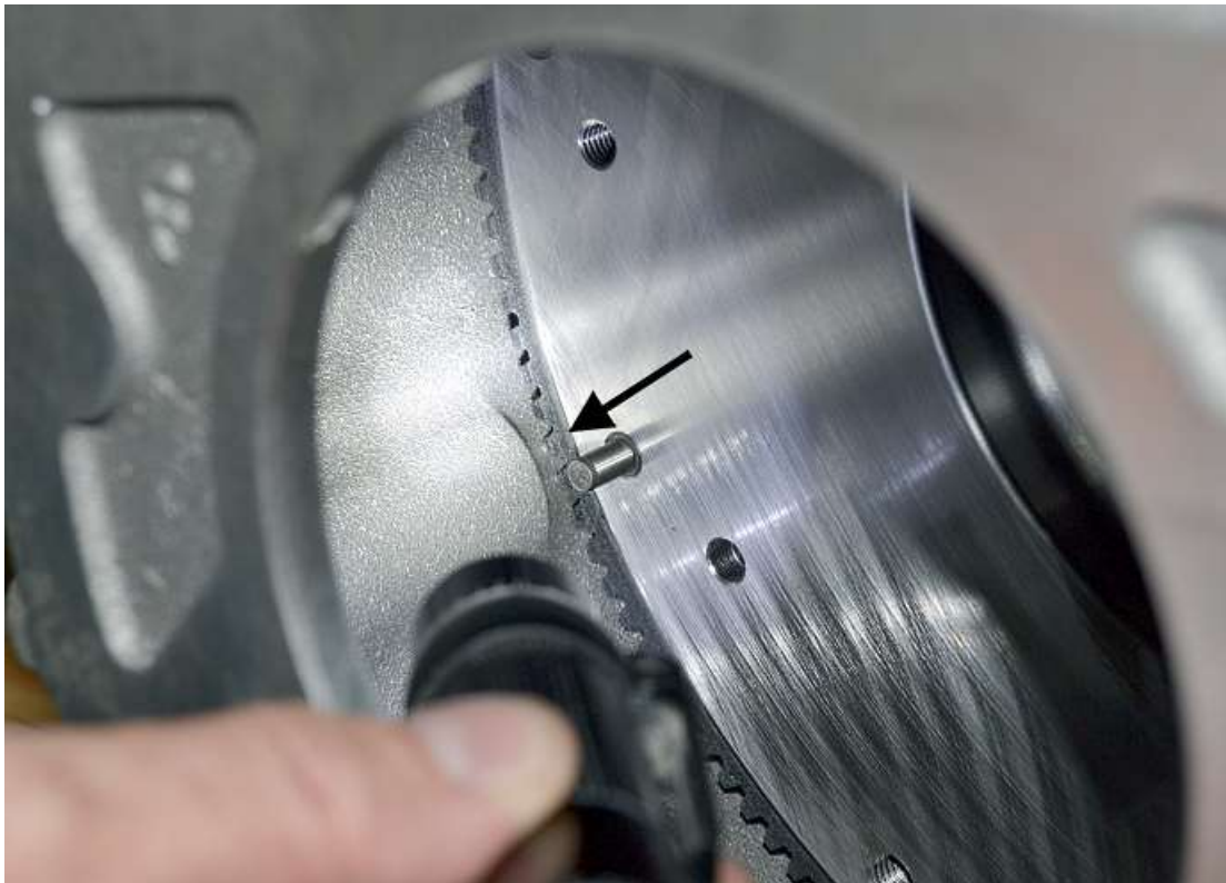
Look inside the bellhousing just above the clutch fork hole or try to turn the engine over using the crank bolt.
