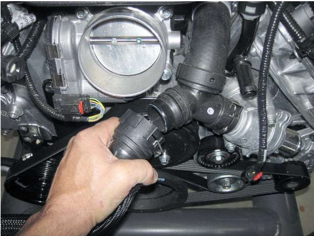
Push the Ford supplied hose onto the outlet under the throttle body.
