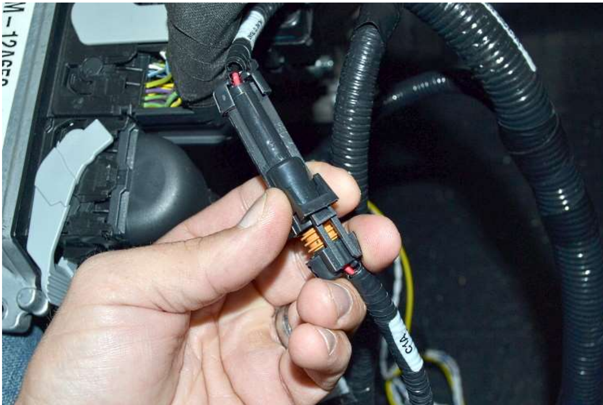
Connect the single wire connector on the transmission harness to the plug on the engine main harness.
