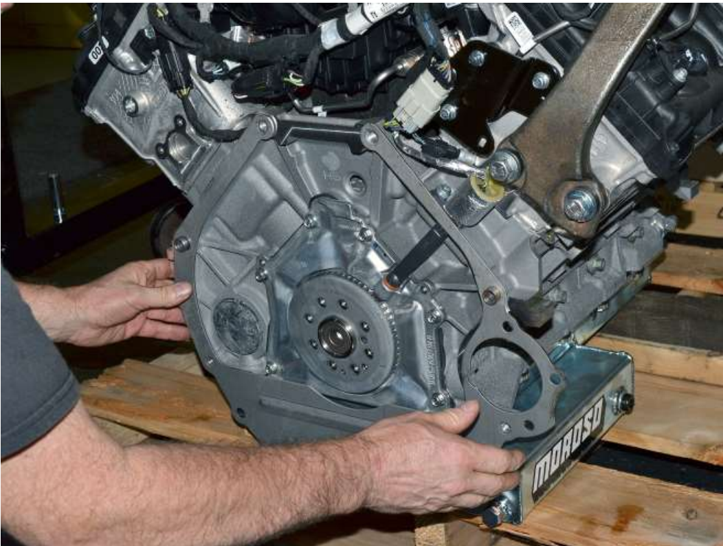
Put the inspection plate on the back of the engine.
