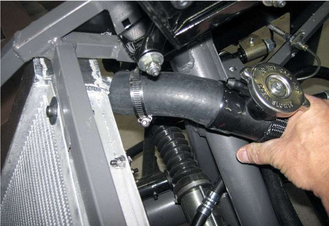
Push the inline filler onto the top radiator inlet making sure to have a hose clamp on the hose.
