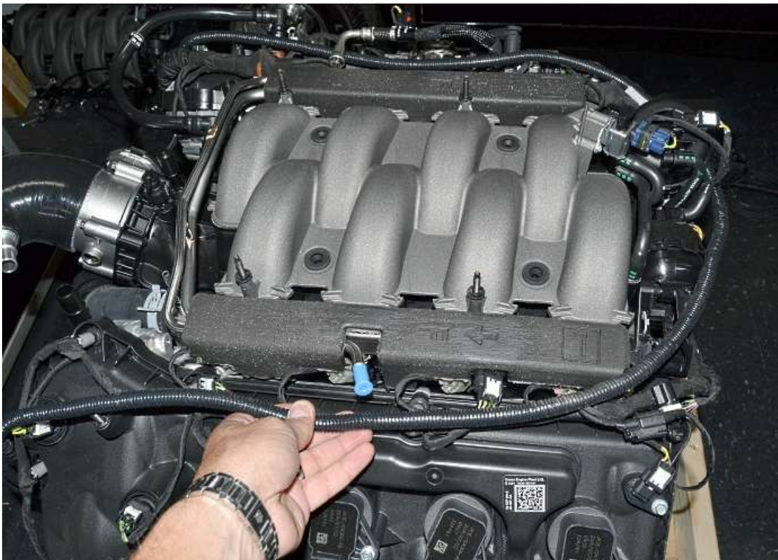
Run the harness leg across to the left side then to the front of the engine on the left side.
