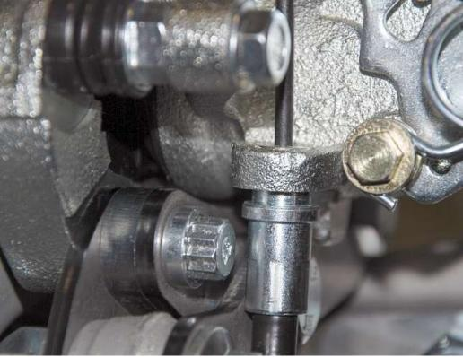
Push the end of the sheath into the hole. The end of the sheath may or may not bottom on the flange. It is normal for the sheath to look like the picture, the end is being held in place and cannot move.
