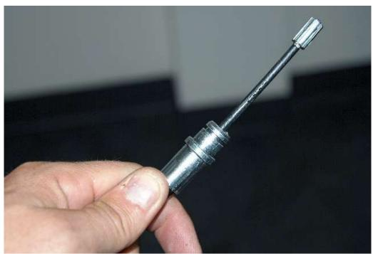
On the end of the Emergency brake cable sheath with no clip on, pull/push the cable so that 3" of cable sticks out of the sheath.
