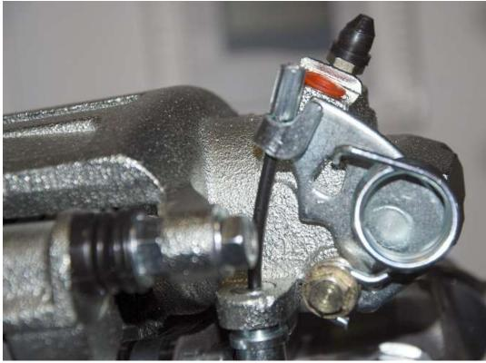
Push the cable so that the end of the cable sits on the spring bracket.
