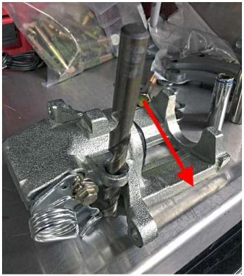
Use a ½" drill bit and run it through the E-brake cable mounting hole then pull it down slightly to oval the hole out.
