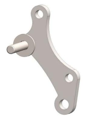
Run the 60mm bolt through the laser cut bracket and ½" washer.
