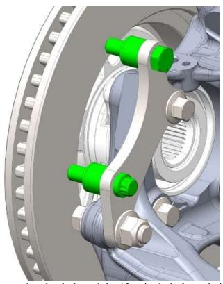
Run the 45mm Hex bolt through the top bracket hole and the 12 point bolt through the bottom followed by the spacers then the shims.
