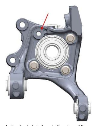
Remove the rear top bolt holding the bearing/hub to the spindle using a 15mm socket and impact wrench.
