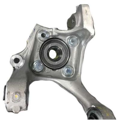
Use a Sawzall to cut the caliper ear off.
