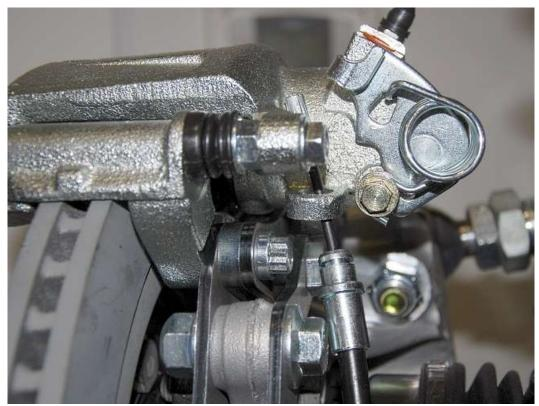
From the bottom, insert the cable through the hole in the brake caliper.
