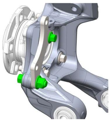
Attach the top bracket bolt to the spindle bearing/hub location and run the larger 14mm bolt from the hub side in. Torque the top bolt to 133 Nm (98 lb-ft) then rotate 45°. Torque the lower bolt to 133 Nm (98 lb-ft).
