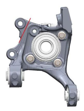
Mark the top brake caliper ear.
