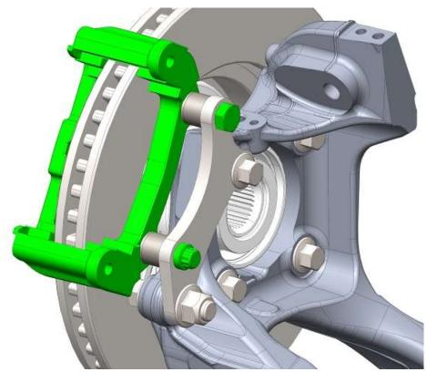
Attach the brake caliper to the bracket. Make sure the bleeder screw is at the top. Make sure the caliper bracket is centered on the rotor. If necessary remove the thin shims.
