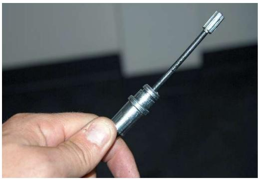
On the end of the Emergency brake cable sheath with no clip on, pull/push the cable so that 3" of cable sticks out of the sheath.
