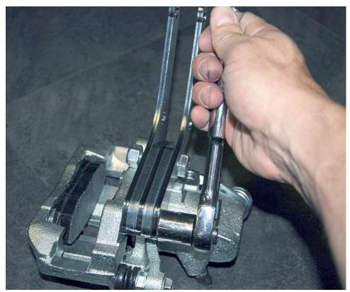
Tighten the front caliper screw using a 19mm socket and ratchet. This will get torqued when the assembly is on the spindle.
