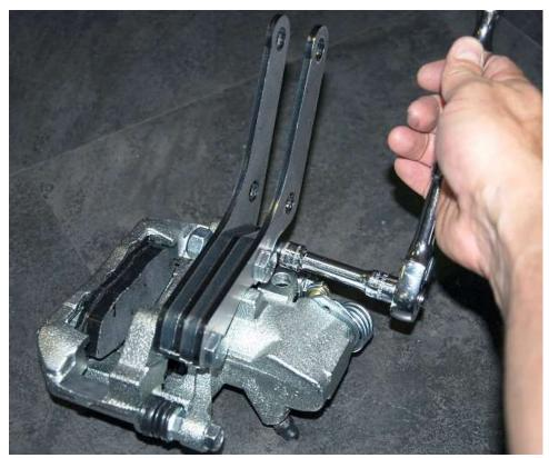
Tighten the rear caliper screw using a 12mm 12 point socket and ratchet. This will get torqued when the assembly is on the spindle.
