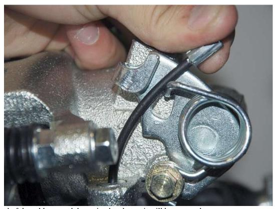
Move the end of the cable around the spring bracket so it will be captured.
