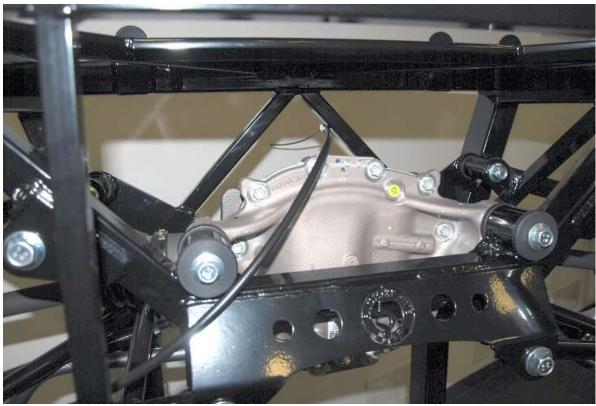
Route the cable up over the center section an to the bracket in the transmission tunnel.
