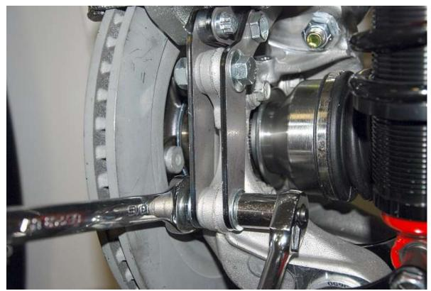
Use a <sup>13</sup>/<sub>16</sub>" wrench, 18mm socket and ratchet to tighten the 14mm bolts.
