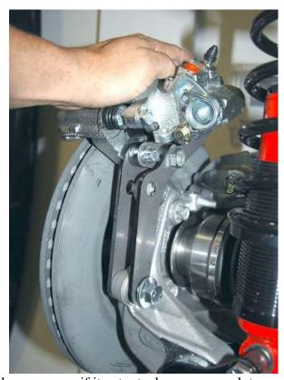
Swing the assembly up over the upper ear, if it gets stuck, use a wrench to spread the brackets slightly.
