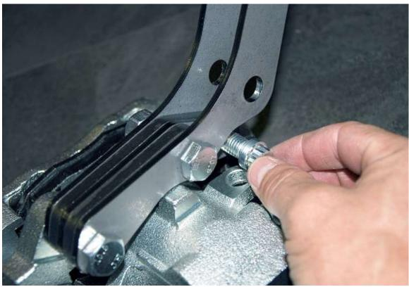
Screw the 12 point 12mm screw into the other caliper bracket hole.
