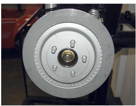
Put the rotor on the spindle.
