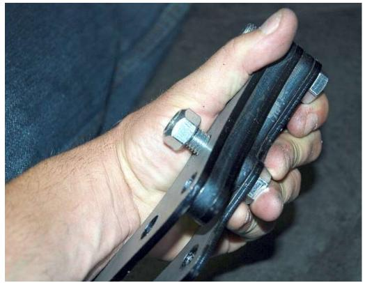
Carefully pick the stack up and put the 12mm lock nut on the bolt in the middle hole.
