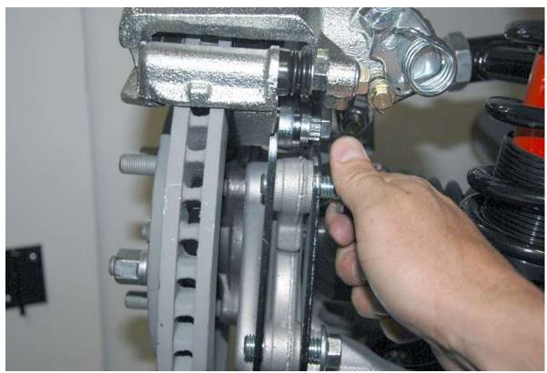
From the inside insert the last 14mm bolt so that 2-3 threads stick through the outside.
