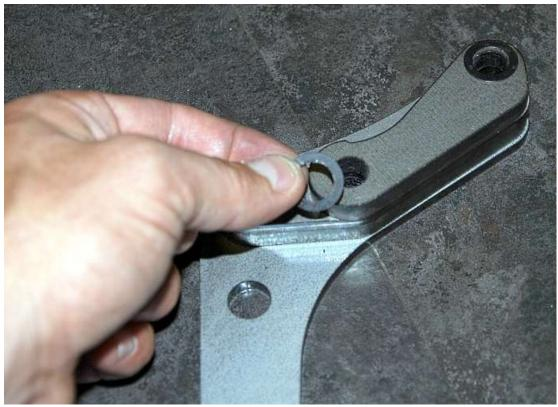
Starting with the outside bracket (16635) first, stack the brackets together as shown in the drawing on the first page making sure to put the shims between the last two brackets.
