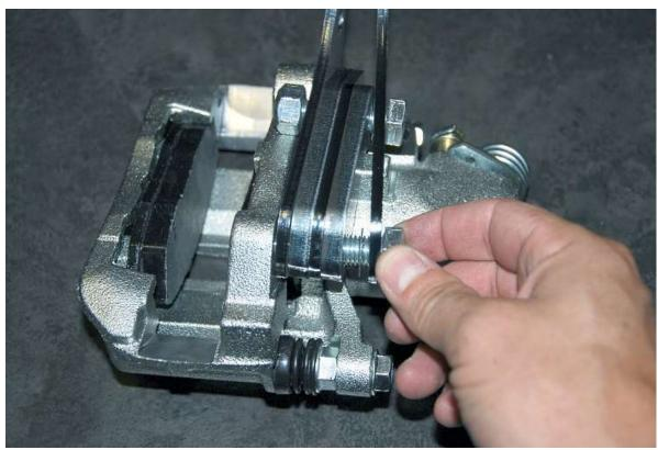
Put the left caliper on a bench upside down with the spring away from you and screw the long 12mm bolt into the caliper bracket by hand.
