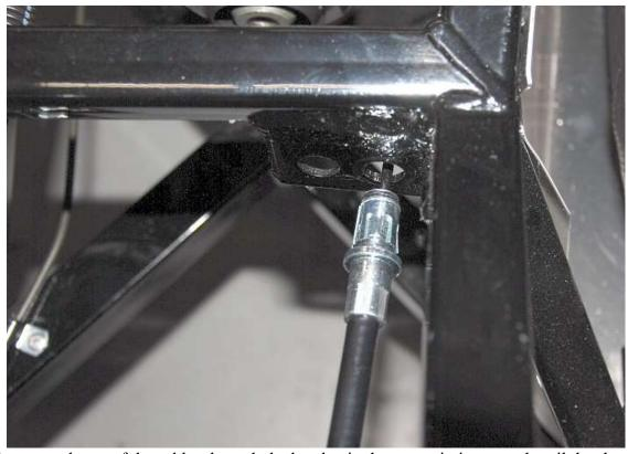
For the Coupe, push one of the cables through the bracket in the transmission tunnel until the sheath end clicks in place.
