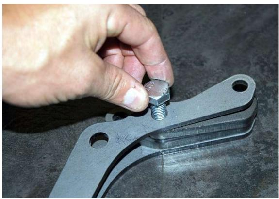
Insert one of the longer 12mm bolts through the middle hole in the bracket.
