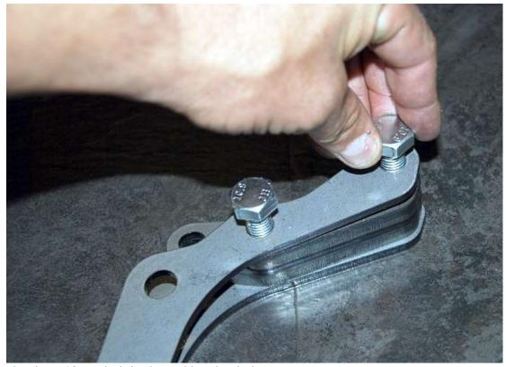
Insert the other long 12mm bolt in the end bracket hole.
