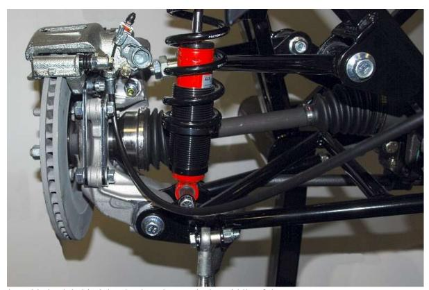
Route the cable back behind the shock and towards the middle of the car.
