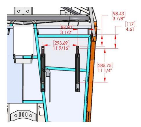
Use the diagram above to locate the rear holes on the cockpit floor Use a  $^5/_{16}$ " bit to drill the track hole locations.
