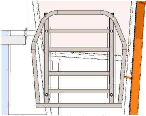
Mark the seat frame for the track mounting holes, the rear holes should be centered on the vertical and horizontal tubes. The front holes should be 11.25" forward of the rear holes. If the tube distance measured earlier was different, modify the locations accordingly.
