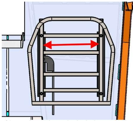
Look at the bottom of the seat and measure between the tubes that the seat track will mount on. The measurement should be  $11^9/_{16}$ " to the center of the tubes. If not, the measurements in the picture below, to the seat belt mount and between the tracks should be adjusted.
