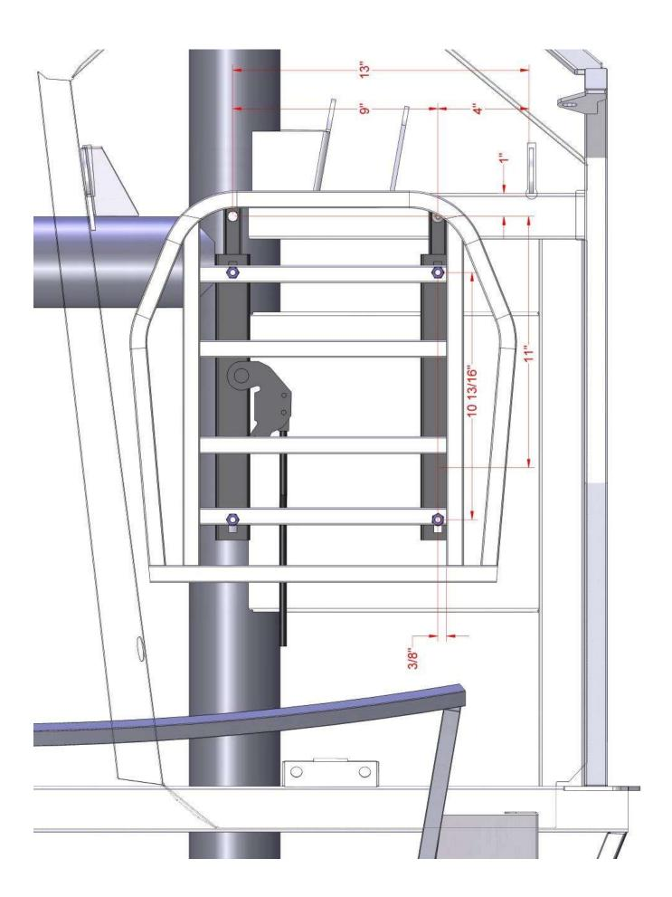
Draw a line on the drivers floor 1" forward from the outer seat harness mount and 13" towards the inside of the car. This is the middle of the 4" round tube which touches the aluminum floor panel and the inner rear seat track mount.
