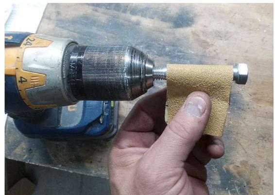
If it is too tight, put the bolt in a drill and run some sandpaper over the bolt.
