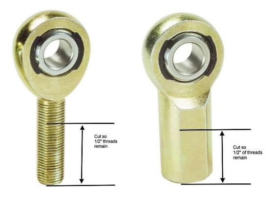
If necessary the minimum length the rod ends and female rod ends can end up are so the threads are  $\frac{1}{2}$ " long.
