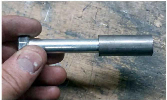
Check the swaybar mount bolt fit in the spacer.
