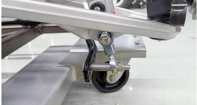
Run the  $7/_{16}$ " bolt through the swaybar, spacer and the rod end.
