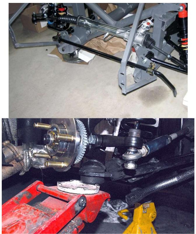
Place the jack under the lower control arm balljoint without hitting the grease fitting.
