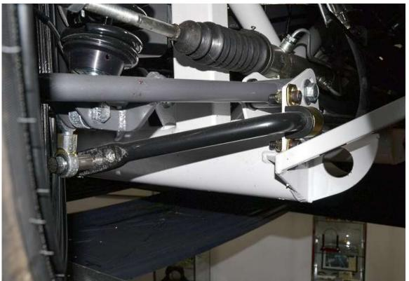
The sway bar should be horizontal or angled down slightly from the bushing to the end. If it is angled down more than  $20^{\circ}$ , shorten more of the rod ends.
