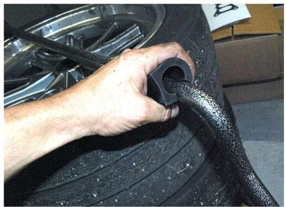
Push the bushings onto the swaybar.
