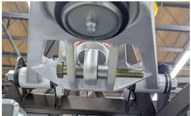
Change the lower shock bolt to the longer  $\frac{1}{2}$ "-13 x3.25" one included with the sway bar and run it from the front of the car towards the back.
