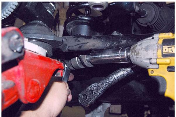
Remove the lower shock mount bolt.
