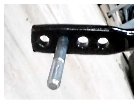
As a starting point, start with the  $2^{nd}$  hole from the end of the bar. If after driving there is too much lean when going around corners, move the bolt to the  $3^{rd}$  hole from the end and retry.
