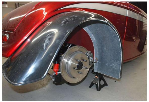
Position the rear fender on the body so it fits tight on the inside, hold it in place with clamps.
