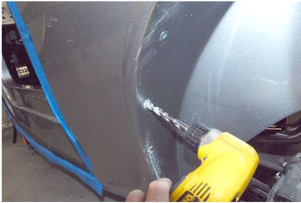
Remove the fender and enlarge the hole in the body to 25/64"
