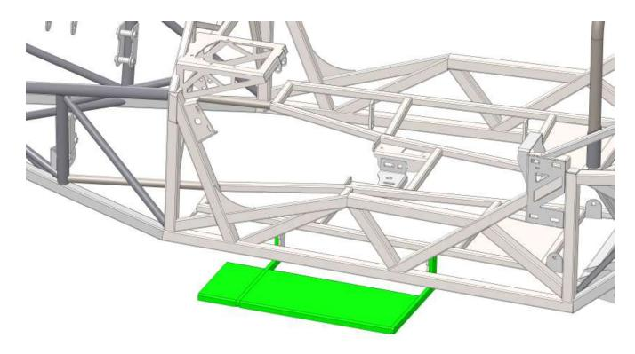
Attach the running board mounts to the frame using the ½" carriage bolts and ¾" socket. Left side shown.
